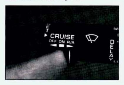
Suppose you set your cruise control at a desired speed and then you apply the brake. This, of course, shuts off the cruise control. But you don't need to reset it. Once you're going about 25 mph (40 km/h) or more, you can move the cruise control switch from ON to R/A (Resume/Accelerate) for about half a second.
